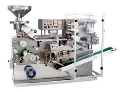
LPH-250 High-speed Automatic Blister Packing Machine is a high-tech blister packing equipment which has gained two advanced patented technologies. It has been rewarded as the provincial scientific and technological achievement product. Its punch frequency is as high as 60-160 times/minute, thus gains a high productive capacity. With higher efficiency and lower cost, this machine provides a new choice for medicine packing in pharmaceutical industry.
