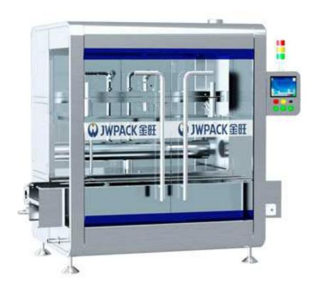
CZ-4Y automatic weighing filling machine consists of linear scale platform (with roller path), chain rod inlet and exit mechanism, fast, slow filling mechanism, material cylinder, weighing control instrument and programmable control unit. The liquid filling scale can meet the needs of automatic weighing and filling of multiple liquids.
