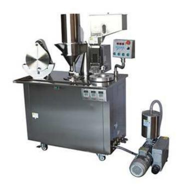
The Semi-automatic Capsule Filling Machine is special capsule filling machine which is suitable for medium &small pharmaceutical factory, hospital preparation lab, etc.
