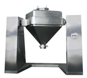
Materials are charged into a closed square-cone mixing barrel, the symmetrical axes of hopper and the axes of rotating shaft form an included angle, materials with different constituents are strenuously rolling over in the closed hopper and producing high shear to achieve the best effect of mixing.
