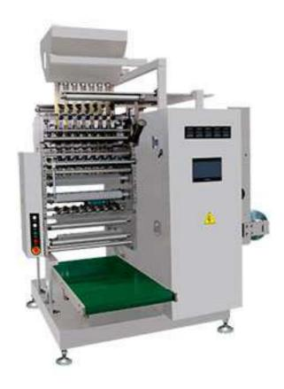
This machine is suitable for pharmaceutical industry, food and cosmetics inductry. Powder, tablets, viscous material can be packed in bag by this machine. It will be well sealing and water resistance for special light and humidity sensitive material. Prevent from gas, ultraviolet rays which is greatly extending the shelf life of material.
