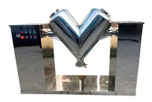
V cone Blending Machine is used for the blending of free flowing solid (powder, granule, etc.) in Pharmaceutical, Foodstuff, Spice, Chemical Industry. The materials being blended are loaded from top feed ports. The recommended loading factor is 40%-60%. Materials being blended are constantly being split and intermixed as the shell rotates achieve a uniform mixture.
