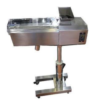
The high-speed tablet deduster model HRD-100A adopts the principle of compressed air purging, centrifugal dedusting and roller deburring and vacuum extraction to clean the powder attaching on the surface of tablet is clean and the edges are regular. It's suitable for high speed dedusting for all kind of tablets. This machine can be linked directly to any type of high speed tablet press.
