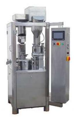
This machine is an intermittent motion and hole plate type filling fully automatic capsule filling Equipment.
