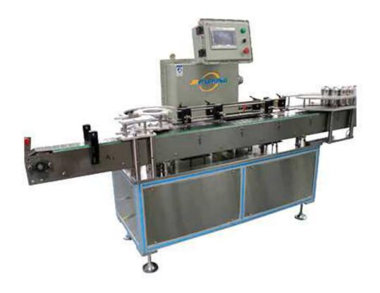
This automatic weighing machine for aerosol filling line, adopted advanced weigh sensor and detecting device, which is controlled and operated by Siemens PLC and Schneider component with low voltage. All electrical appliances have been placed in explosive-proof cabinet.
