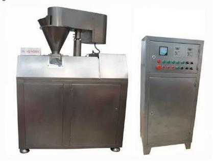
GL dry extrusion granulator directly makes dry powder degassed and pre-shrunk. It exerts a force on rollers through hydraulic pressure for extruding out sheets, and then makes needed granules through smashing and granule integrating. This high speed granulator is widely used in chemistry, pharmacy, food and other powder-processing industries.
