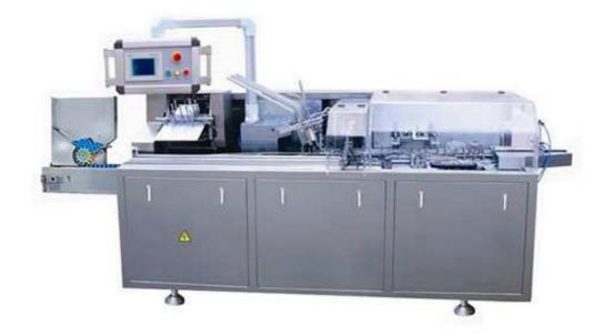
This machine is applicable for encasing ointment, injection and vial etc automatically. The working process is product conveying, leaflet conveying (1-4 fold), carton opening and conveying, box and leaflet encasing, meanwhile finish auto batch coding and carton sealing. (Hot melt glue device as option)
