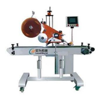
Automatic plane labeling machine, suitable for flat plane labeling machine, especially suitable for paper side, top, bottom, machine body is small, can be used in narrow places, can also be used in wiring, can add barcode printer, integrated with the supervision system.
