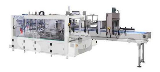
This machine shapes the cartons automatically and closes their bottoms flaps within hot glue.
