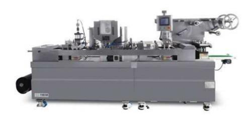
Automatic coffee capsule packing machine can make the coffee cup by heating the polypropylene sheet on and precise dragging it by the servo traction to the next station for feeding filter layer, filling coffee, powder, and feeding the second filter layer, sealing and punching. The final products will be outputted through conveyor belt.
