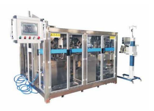
HB25-PE automatic bagging machine mainly used for PE bag (polyethylene bag). It has fully bagging functions, such as weighing, filling and bag sealing. Stainless steel structure suits a lot of industry, such as food packaging, chemical packaging, pharmaceutical packaging, etc. The speed can be up to 1200 bags per hour.
