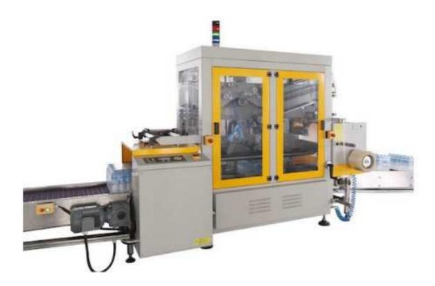
This carry handle applicator is to apply carry tape on shrink film product, carton packer product or other packed product. This new carry handle applicator machine provide convenience to customer and speed can reach 25 packer per minute.
