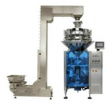
It can fully complete process including Combination-weighing, product filling, film forming, bag sealing, punching, printing, and counting.
