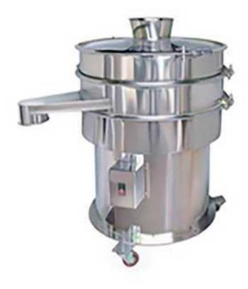
Vibro Sifter is used for screening, sieving, grading for solid-liquid separation, process to separate the desired elements and the undesired elements from the combination of solid to solid (where two solids are generally having different properties) and solid to liquid material. It used in various industries such as Pharmaceutical, Chemicals, Cosmetics, plastics, paints, plastic, minerals, rubber compounds, metal powders, detergents, pesticides and fertilizers, dyestuff and pigments
