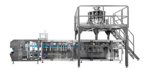
By using a variety of heat sealable multi-layer complex film, our doypack machine series horizontal FFS packaging machine is designed for packaging doypack (standup pouches) and is fully automatic system for pouch forming, filling, sealing. Equipped with our filling or dosing system, customer can fill various products: powder, liquid or granule.
