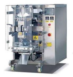
1. Imported PLC computer control system with human-machine interface; touch screen is simple and direct-viewing in operation;
