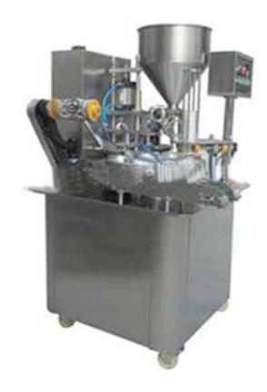
This machine is mainly used to fill liquid such as Water, juice, Yogurt, etc or Semi-liquid such as Paste, jelly, ice cream, pudding, powder, jam, porridge, ketchup, etc.
