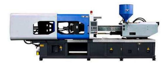
Pet preform injection molding machine equipped with high performance servo motor controlling system, the machine's output power can vary in accordance with the loading changes, which reduce energy consumption and noise. The motor rotates at lower speed in holding pressure stage, an doesn't work in cooling time.
