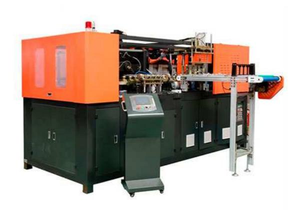
Automatic China PET jar blowing machine J4 is specialized euipment designed for wide neck PET jars. It is high automatically, wide versatility and easy operation. It is especially suitable for the production of neck 50-180mm. J series bottle making machine is precisely positioned and adopts advanced microcomputer PLC control system, which is more stable.
