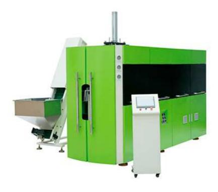
WBB-4SS 4cavity automatic PET plastic bottle blowing machine with 3 servo motor (moving perform and clamping system and stretching system) output 7000 bph, which is suitable for blowing any shape of PET bottles, such as carbonated bottles, water bottles, juice bottles, oil bottles, etc.
