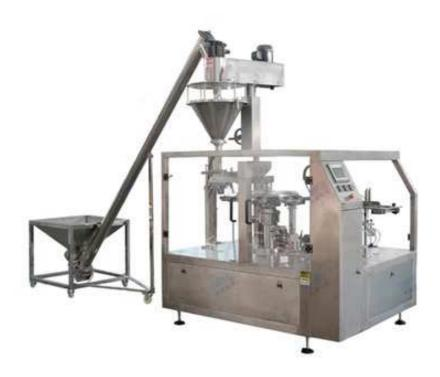
The doypack filling machine can be applied to the packaging of liquids, hot pot bottom materials, pellets, sauces, powders, puffed foods, daily necessities, hardware accessories, medicines, fertilizers, feeds, irregular blocks, strips and other materials. It only needs to be selected according to different materials. Different metering devices are sufficient.
