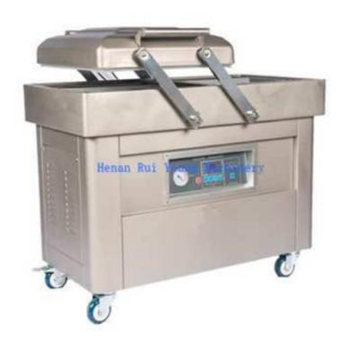
This equipment has a wide range of applications. Suitable for all kinds of plastic composite film bags or aluminum foil composite film bags. it can be packaged in a vacuum bag, which is universal for both large and small bags, suitable for solids, granules, powders.
