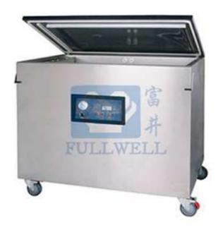
CE-800/DZ series single chamber vacuum packaging machine can finish the whole programs of vacuum extraction, sealing, cooling and exhaust automatically. The products after packing can be prevented from oxidation, going mould, insects or getting damp, thus can be kept fresh for longer time.
