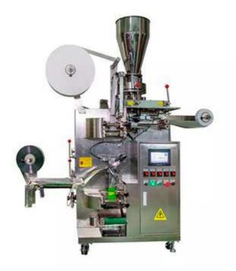
XH-68 small tea packaging machine is a fully automatic tea bag filling and sealing machine with mature technology. It is mainly composed of a rectangular filter tea bag-making machine and an outer envelope sealing machine. The inner dip tea bag can be packed with or without thread and label.
