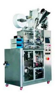
This packaging machine is suitable for drip coffee bag with outer envelope, and it is available with coffee, tea leaves, herbal tea, health care tea, roots, and other small granule products. The standard machine adopts the fully ultrasonic sealing for inner bag and heating sealing for outer bag.
