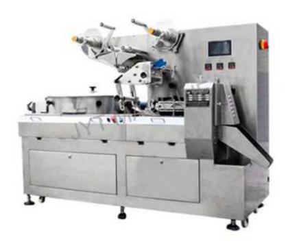
Suitable for granular package of wafer-shaped, spherical, fine-circular, round-shaped, cylindrical candies and other solid objects with regular shapes.
