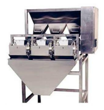
The Tridyne F-206 Series offer the best in high speed filling and packaging. From 20-40 weighments per minute, this machine is a work horse. This series uses Allen Bradley PLC controls with a user-friendly touch screen operator interface. Controls can be set up with network capabilities and many other options and features are built in based on customer requirements. Available in the F-206, F-206-X, and F-206 Super-X series in several different models, able to serve copious purposes.
