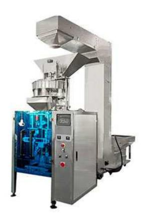
Volumetric Measuring Cup Packing Machine with Hoist can automate the packing of granular, powder, flake, strip and other materials. It is suitable for paper, cellophane, aluminum foil and other heat-sealed laminated packaging materials. You can choose one of the three packaging forms: back sealing, three side sealing and four side sealing. This machine is suitable for packing melon seeds, corn kernels, soybeans, peanuts, nuts, granulated sugar and other small granular materials for metering.
