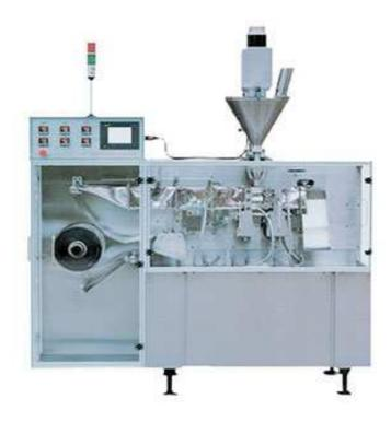
The machine is operated by PLC programmable control system, which can realize filling conversion of powder, granule, water and viscous liquid. According to the need to achieve three or four edge sealing. It is an ideal small dose filling machine in China. The parts in contact with materials are made of high quality stainless steel, which can be easily removed, cleaned and maintained. The machine conforms to GMP requirements.
