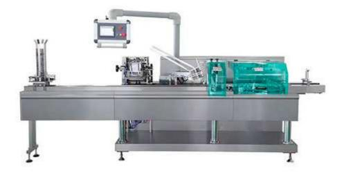
This medicine cartoning packing machine mainly includes seven parts: medicine in-feed mechanism, pharmaceutical in-feed chain part, carton suction mechanism, pusher mechanism, carton storage mechanism, carton shaping mechanim and output mechanim.
