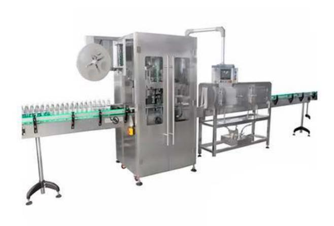
Shrink Sleeve Labeling Machine has flexible film shrink sleeve labels placed onto bottles using a sleeve applicator or sleeve labeler. The sleeves are then held in place by shrinking them using hot air or steam from a heat tunnel.
