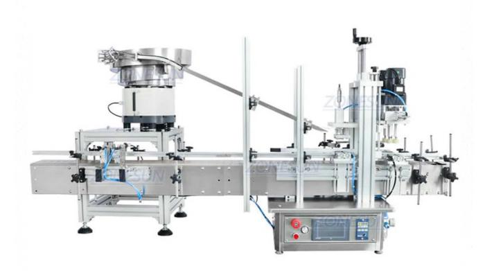
This tabletop automatic capping machine tighten bottle caps by screwing 4 rubber wheels. This kinds of capping method makes it has wider application range. It is suitable for spray bottles, dropper bottles etc. It is equipped with vibratory bowl, which can arrange bottle caps and feed bottle caps automatically, helps you save labor.
