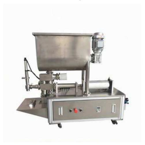
This machine is mainly designed and produced for the sauce distribution of the food industry. It is especially suitable for chili sauce, bean paste, peanut butter, sesame paste, jam, butter hot pot bottom material and red oil hot pot bottom material with granules and high concentration in the seasoning. Filling of viscous sauces with other substances.
