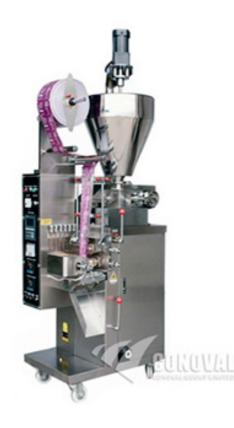
It is suitable for automatically packaging of viscous products with free-flowing such as tomato sauce lotion noodle jam, edible oil, meat jam and broth. The processes of bag making measuring, filling, sealing, counting and hot pressing codes can be done automatically. Packing material include several kinds of heat-seal lamination, such as PET/plated AL/PE, PET/PE, NYLON ...etc.
