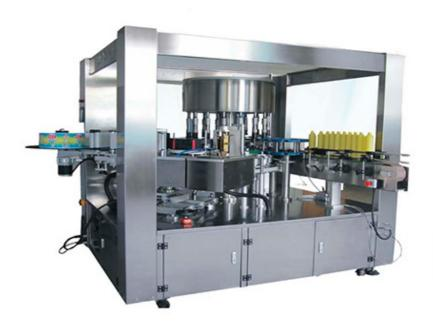
The Automatic Rotary Hot Melt Glue Labeling Machine is suitable for sticking the continuous rolled labels, using local gluing methods in small glue consumption and low running costs. It's widely used in round bottle high-speed labeling for Food and beverage industry, pharmaceutical industry, etc.
