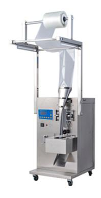
The 300ML pneumatic liquid packing machine produced by JD is suitable for the quantification, weighing, filling, packing and sealing of purified water, milk, juice, soy sauce, edible oil, olive oil, alcohol liquid, seasoning water, brown sugar water, chili oil, red oil, peanut oil, soybean milk and other liquid products.
