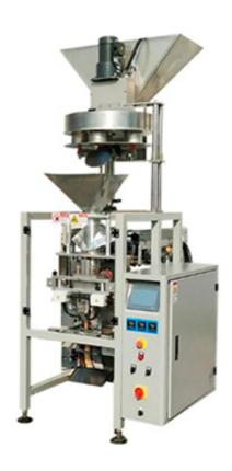
The machine is mainly used for packaging granular products, such as sugar, salt, coffee beans, rice, beans, peanuts, melon seeds, grains, grains, nuts, chocolate beans, cereal, tea, washing powder, desiccant, etc.
