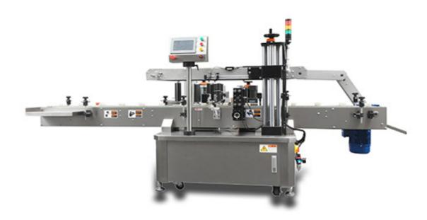
Process flow: feeding  $\rightarrow$  differential splitting  $\rightarrow$  synchronous correction  $\rightarrow$  labeling  $\rightarrow$  secondary smoothing  $\rightarrow$  finished product  $\rightarrow$  next process
