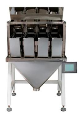
The four-head linear weigher is an advanced, high-tech weighing and packaging system that helps to deliver precise measuring and packing for various products. It has four separate weighing heads situated linearly with each able to independently measure or dispense product into containers meant for packaging.
