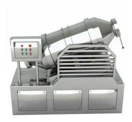
Two-dimensional Mixer is suitable for mixing of dry granule materials in pharmaceutics, chemical and foodstuff industries, especially for those in high tonnage.
