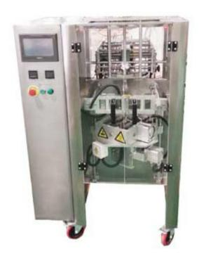
This irregular shaped packing machine is used to pack products into irregular shape sachet, like round shape, hand shape, bottle shape and leaf shape and so on. It's widely used in pharmaceutical, food, cosmetic, chemical and other industries for packing powder, granule, liquid, sugar, pill and other products.
