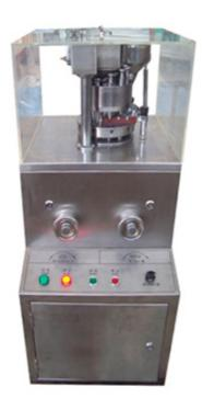
ZP-10EU rotary tablet press is a new generation product by our factory, it's suitable Use the EU standard B or D tooling, and this machine is a single roller continuous automatic tablet press for pressing various kinds of different shape tablets and plain tablets, such as round tablet, irregular tablet and carved tablet etc.
