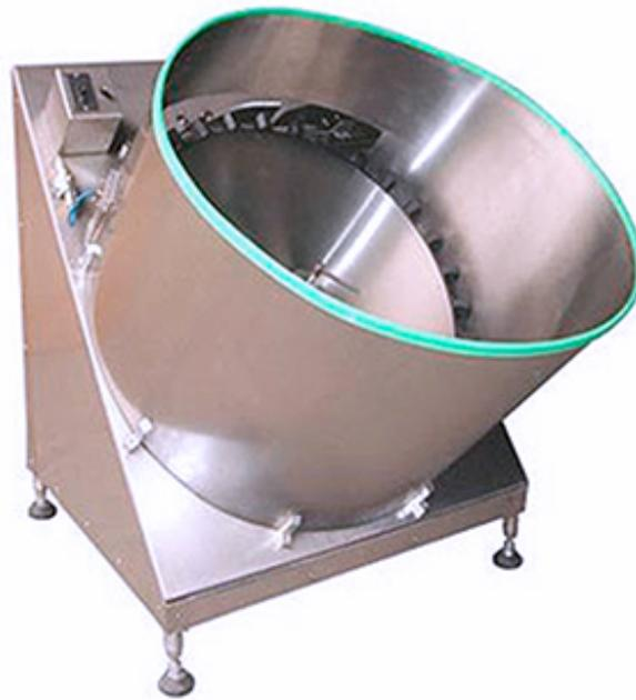
SLP sorts round, rectangular and square bottles automatically and places the containers on a conveyor at speeds up to 100 cpm. This unscramble adopts electronic timing system. The operation is easy and stable. It is useful widely in the pharmacy, food & beverage, cosmetic & personal care industries.
