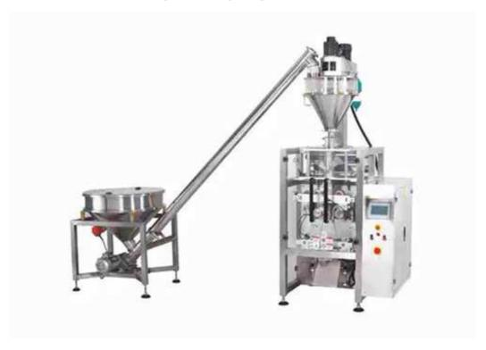
Packaging materials: polyester/polyethylene, polyester aluminized polyethylene, polyester aluminum foil polyethylene, paper polyethylene, nylon and other heat sealable composite materials.
