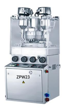
This model is to press the various kinds of granular materials into tablets, with the most outstanding advantage of being able to produce irregular tablets with wide different geometrical shapes, such as double layer tablets, ring like tablets and double side engraved tablets.
