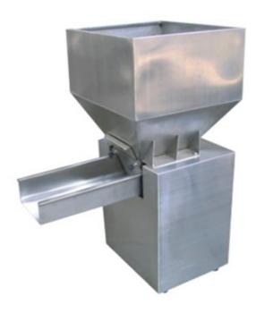
The Vibration Feeder adapted electrical magnet principle as power, using the vibration to transfer the material to the buckets of the bucket elevator. The power is electromagnetism oscillator which is stable, gentle and fast.
